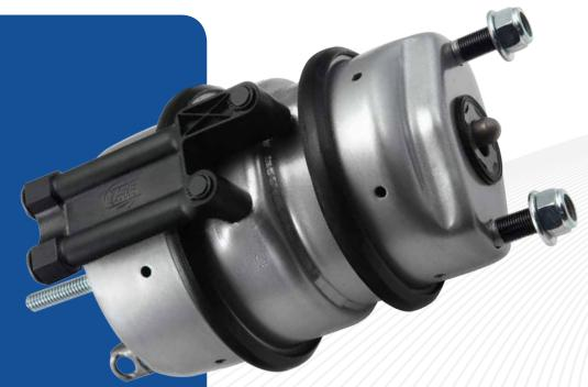
TSE innovated the double-diaphragm HOT (High Output Technology) chamber used worldwide for disc brake applications. Now TSE has taken disc brake actuators to the next level with the ultimate in product durablity and corrosion resistance.
