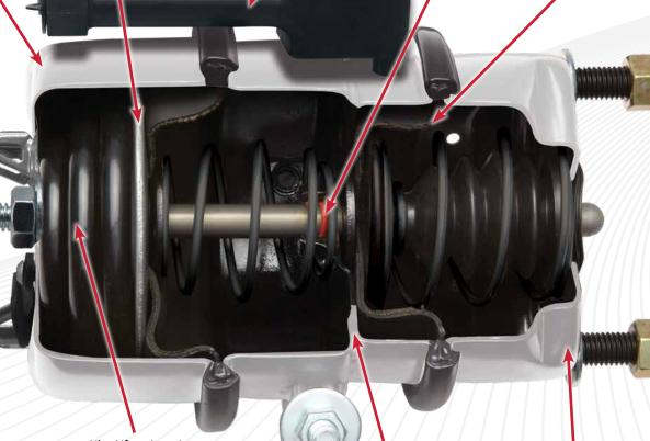
UltraLife main spring adds a proprietary base coating in addition to TSE's multi-stage coating system for the ultimate in corrosion protection.
